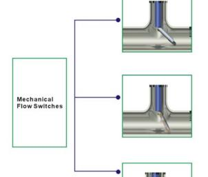
Detect the flow mediums by the swing amplitude of themechanical paddles or probes.
