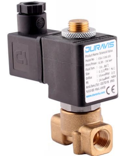
For ESV 107 1: Inlet (Body) 2: Outlet (Body) 3: Exhaust (Enclosing Tube) De-energised: 1-2 Energised: 2-3
