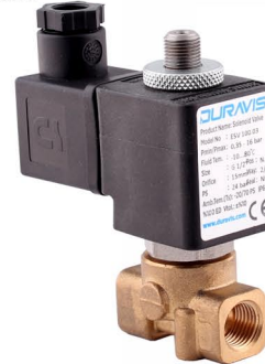
For ESV 106 1: Inlet (Body) 2: Outlet (Body) 3: Exhaust (Enclosing Tube) De-energised: 2-3 (Exhaust) Energised: 1-2
