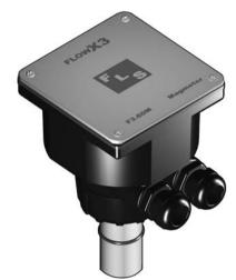
The NEW FLOWX3 F3.60M & F3.63M Insertion Magmeters are suitable to measure flowrate in both metal and thermoplastic pipelines. No moving mechanical parts and the high quality materials allow the measurement of liquids where suspended solids can be present or of abrasive liquids as long as they are conductive and homogeneous.
