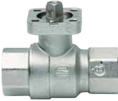
Ball valve, full bore, female/female, with DIN ISO 5211 connection for actuator, nickel-plated.
